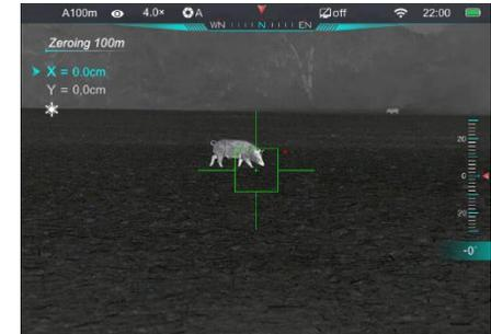
impact. Rotate clockwise to move the reticle right or down, and rotate anticlockwise to move the reticle left or up.
