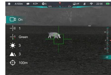
select recording option and press the **Controller (4)** to turn on and start a video recording.
